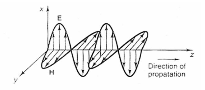
**E**- and **H**-field vectors for a plane wave propagating in *z*-direction
